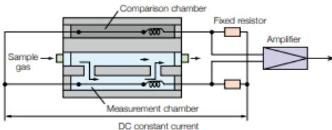
Because the thermal conductivity is different among gas components, when there is a change in the concentration of the component under measurement, the thermal conductivity of the sample gas will change to affect the temperature of the platinum wire. The analyser uses the temperature change to determine the gas concentration.
