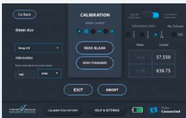
Select channel, cuvette and extraction ratio.
